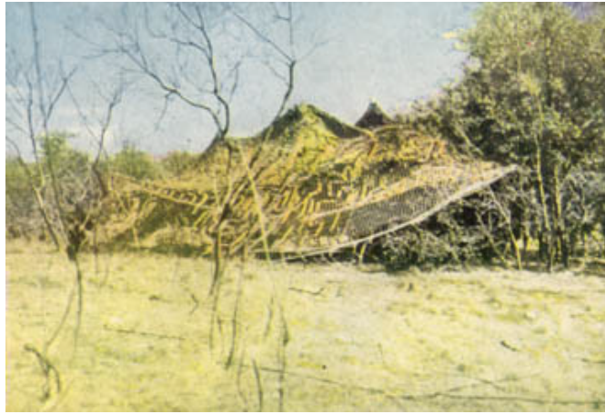
FIGURE 52. A well-draped vehicle. Scrub has been used around the edges of the drape to break up the shadow made by the drape.
